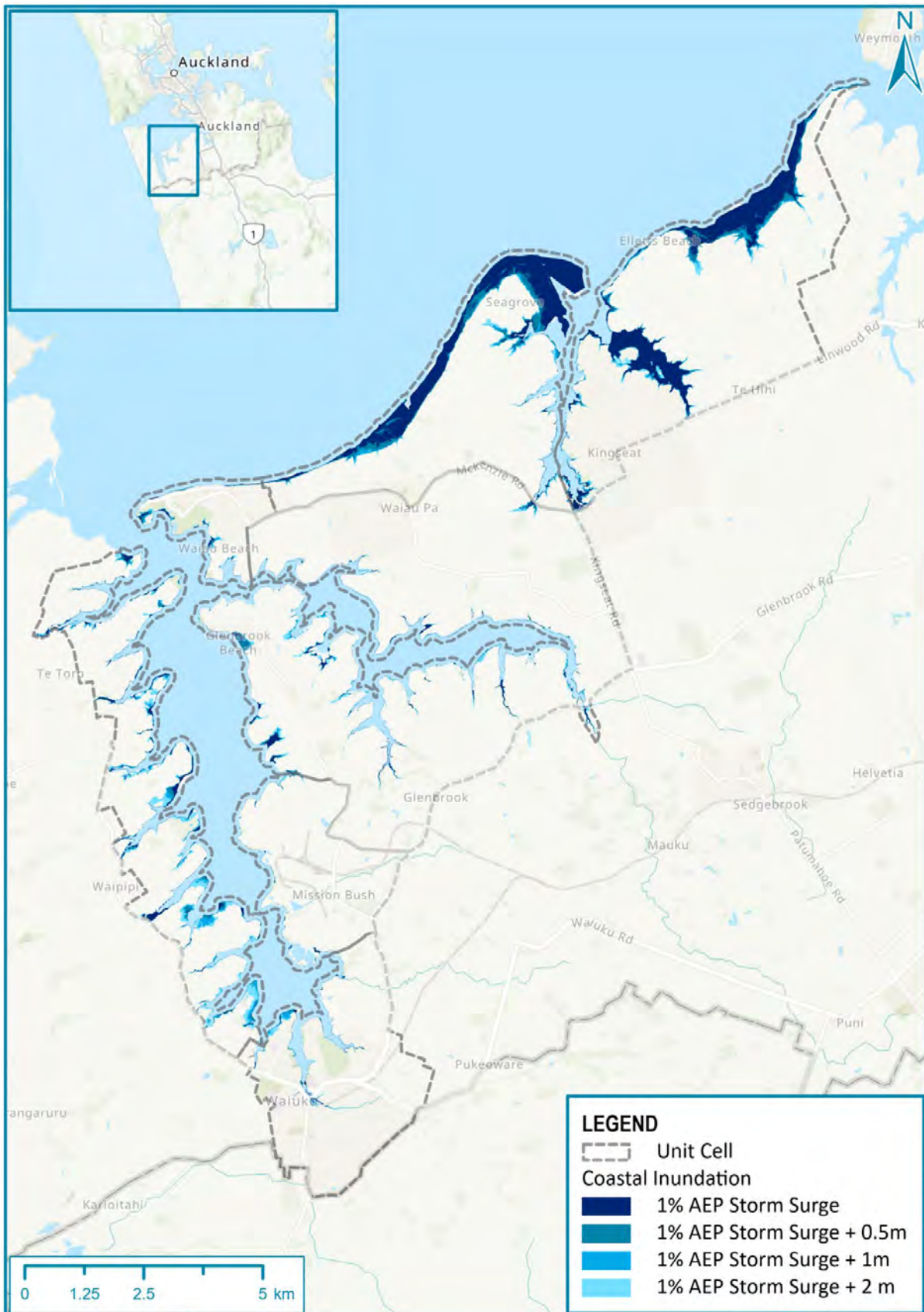
Figure 2-7: Coastal inundation for 1% AEP storm surge for present day and with 0.5 m, 1 m and 2 m sea-level rise.
