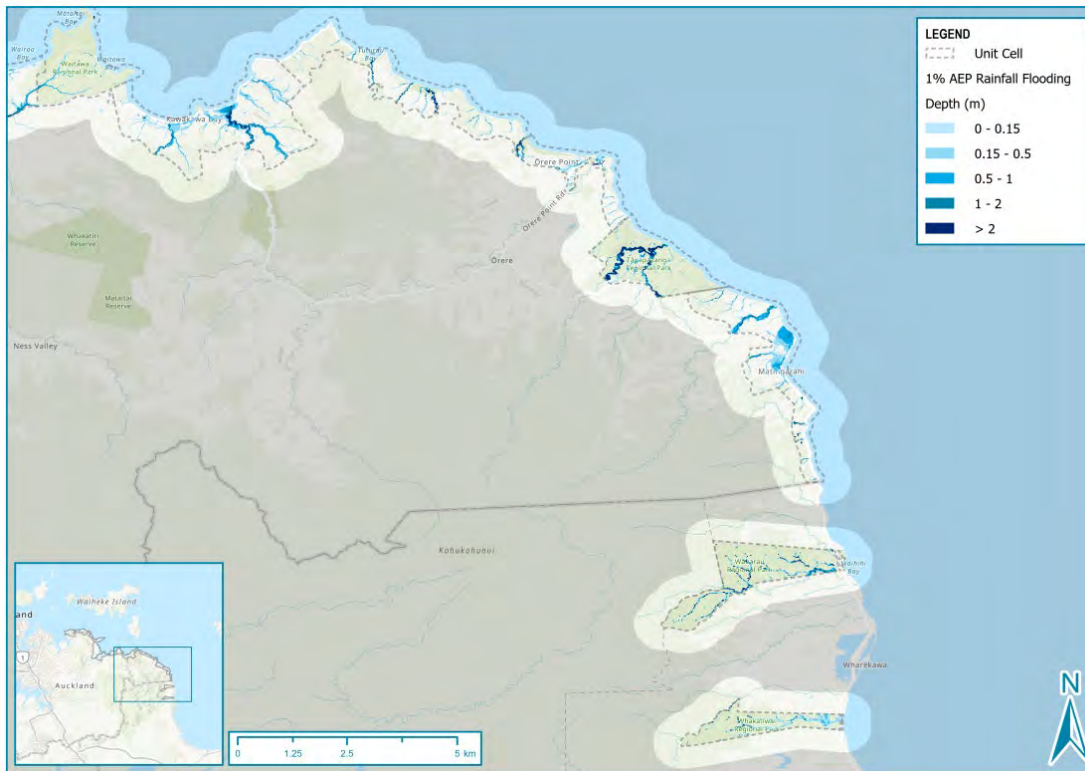
Figure 9: Waitawa Regional Park to Whakatīwai Regional Park Rainfall flood extents and depths for 1% AEP event and the maximum development scenario (2 of 2)
