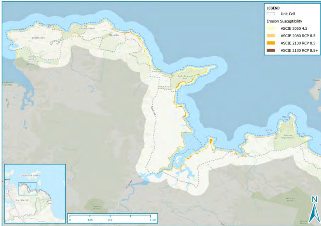
Figure 6: Beachlands to Waitawa Regional Park coastal erosion susceptibility for 2050, 2080 & 2130 considering RCP4.5 and RCP8.5 emission scenarios (1 of 2)
